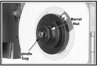
Figure 29. Component identification.
